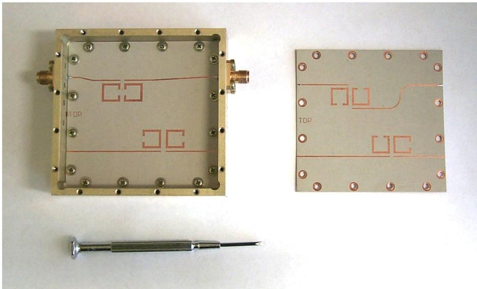
Figure 11: Boards to test resonator coefficients
