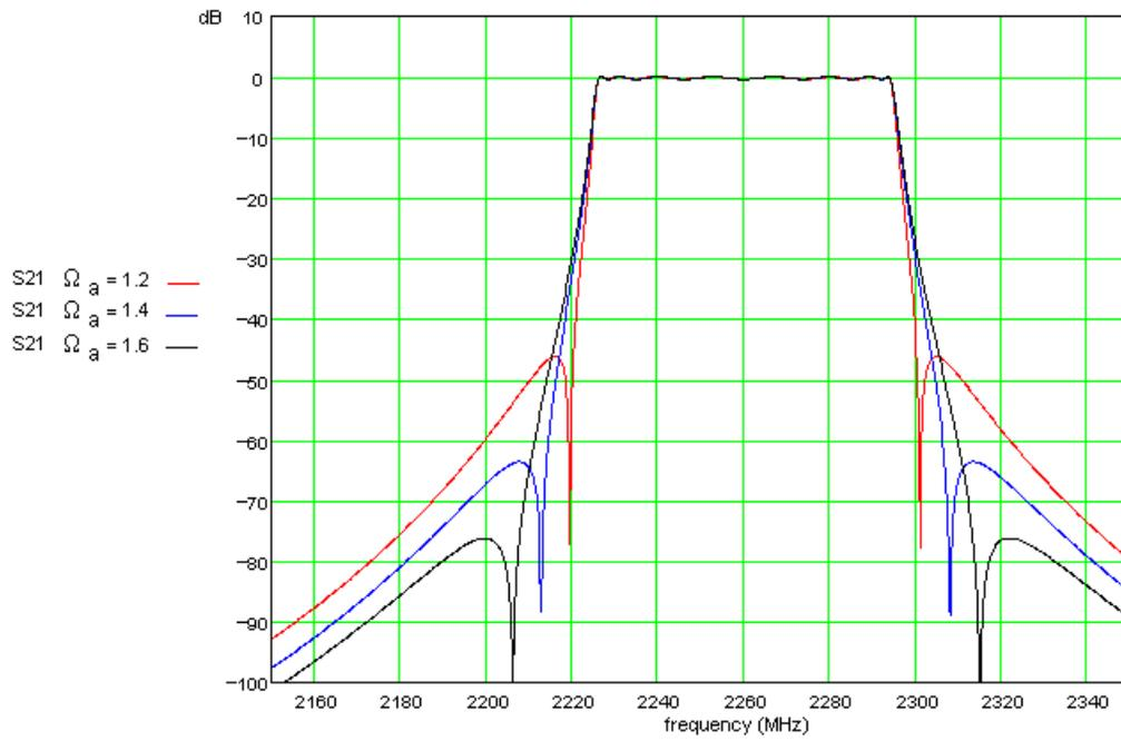
Figure 3: Variations in filter response due to changing its order and  $\Omega_a$
