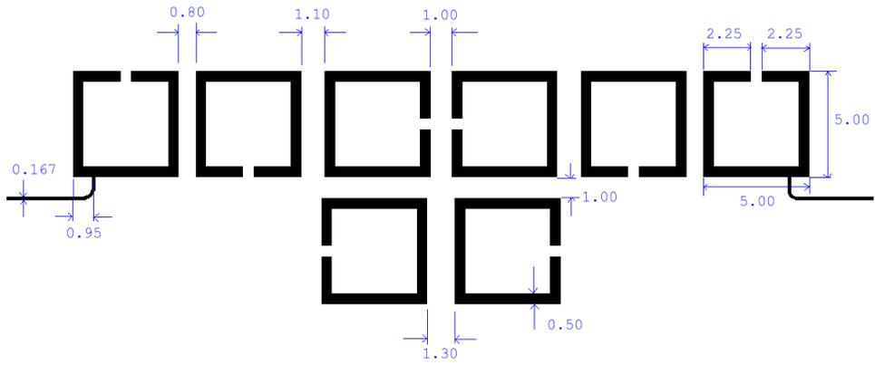
Figure 14: HTS filter layout (dimensions in mm)
