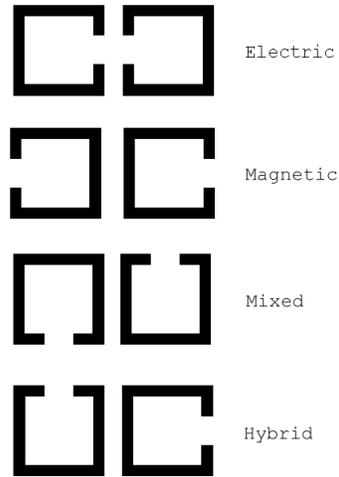
Figure 4: Possible resonator couplings
