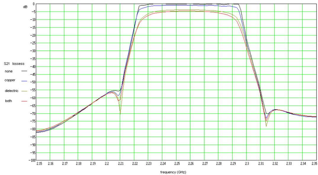
Figure 13: Loss mechanisms
