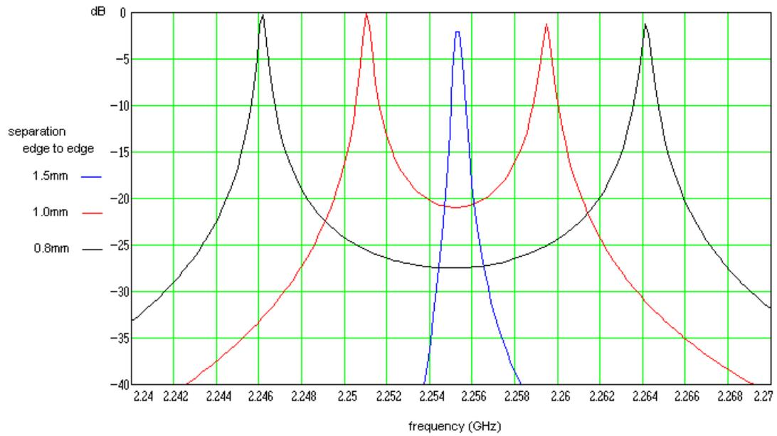
Figure 5: Filter response *vs* distance between coupled resonators
