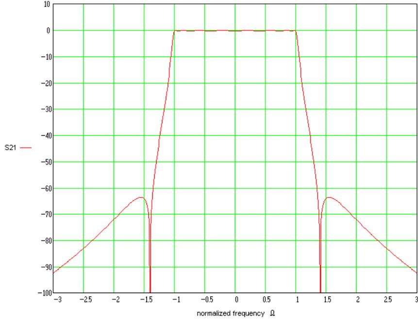
Figure 1: 8-pole quazi-elliptic filter ideal response
