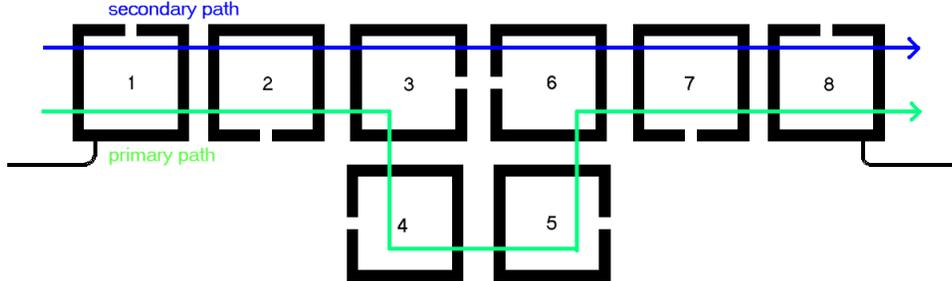
Figure 2: Primary and secondary signal paths
